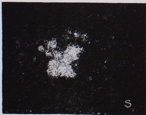
Phot. 5. a — collomorphic aggregate of hydrated iron oxides containing an inclusion of elementary sulphur. Electron absorption image. Magn. \times 1000 . b — distribution of Fe, c — distribution of S
